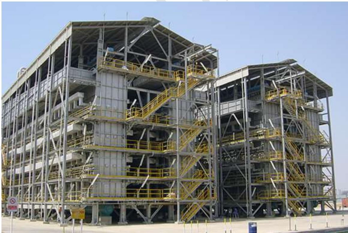
**Figure 17 - Methane Steam Reforming Assembly.** *Source: Haldor Topsoe A/S*
