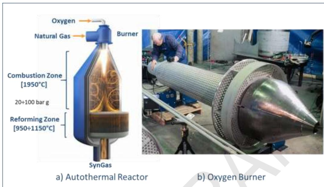
**Figure 19 - Autothermal Reformer.** Source: Haldor Topsoe A/S
