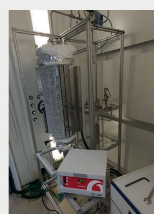
Reactor used for chemical looping reforming of methane
