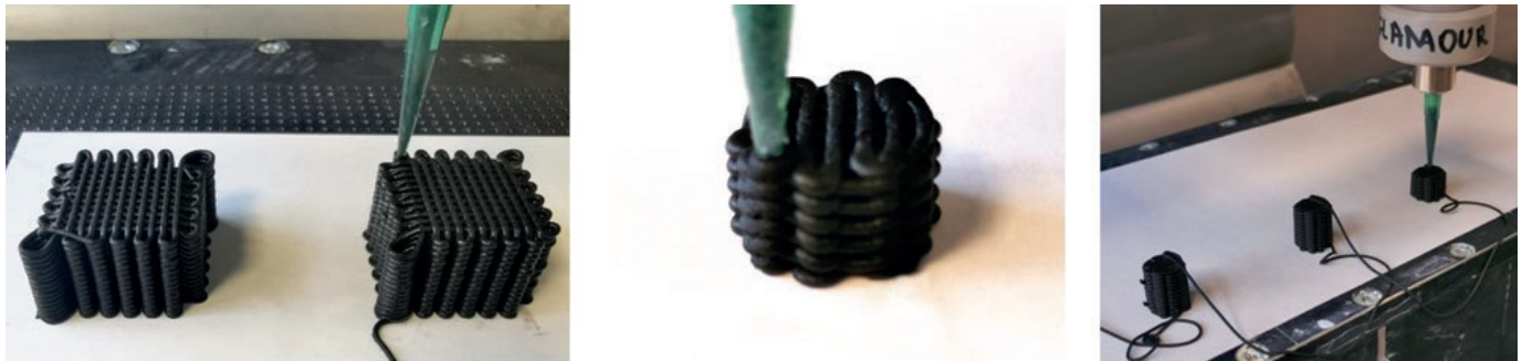
First 3D printed GLAMOUR catalysts produced by VITO
