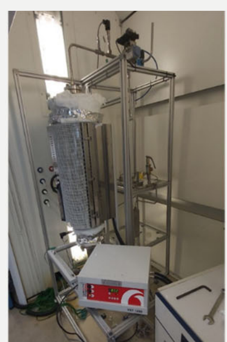
Reactor used for chemical looping reforming of methane
